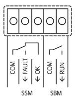
SSM: Collective fault signal (NC contact in accordance with VDI 3814, load capacity 1 A, 250 V ~)
