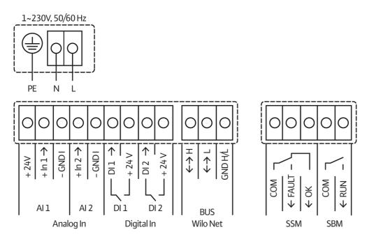
SSM: Collective fault signal (NC contact in accordance with VDI 3814, load capacity 1 A, 250 V ~)
