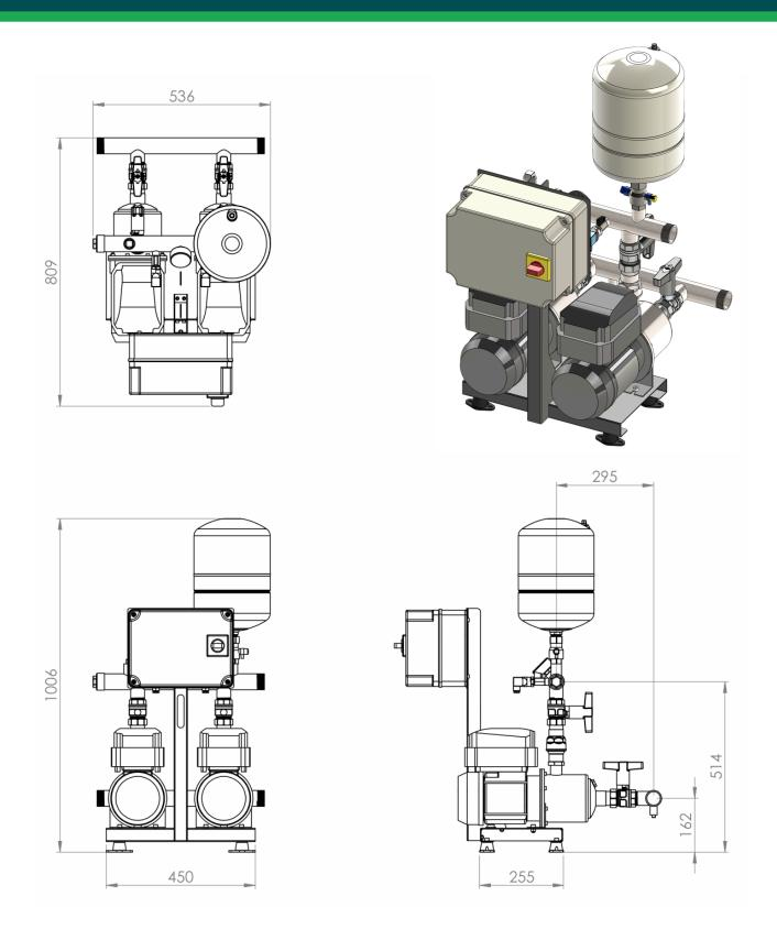
NOTE: The pressure vessel & FlowThru valve are supplied loose along with a cap. They should be fitted to the closest connection to the outlet, dependent upon which end of the discharge manifold is capped off.
