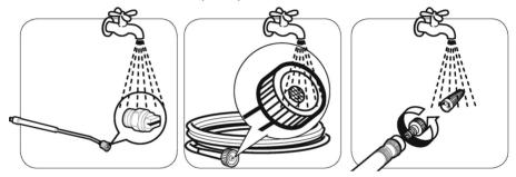
Rinse the nozzle, hose connection and water filter carefully under running water.
