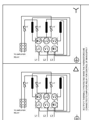
IEC 60921-11 THERMALLY PROTECTED WHEN THE THERMISTORS ARE CONNECTED TO THE RELAY FOR CONTROL OF MAIN SUPPLY
