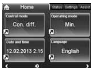
Fig. 19 Example of main display on a TPE Series 2000 with advanced control panel
