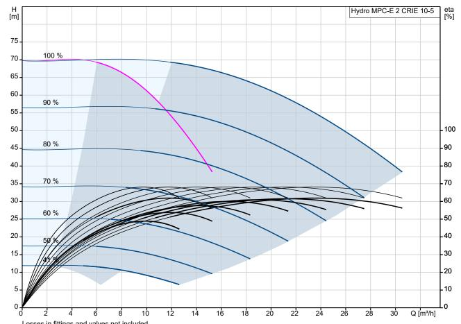
Losses in fittings and valves not included Pumped liquid = Water Liquid temperature during operation = 20 °C
