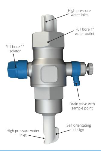
Global Water Solutions' FlowThru™ inline adaptors are ideally suited for constant pressure systems such as hot and cold booster systems controlled by variable frequency or variable speed drives (VFD/VSD). The FlowThru™ inline adaptor diverts the water through the tank while the pump is running, eliminating the risk of stagnant water and reducing the risk of waterborne bacteria such as legionella. This constant flushing ensures the freshest water in the tank.
