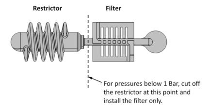
To change the flow restrictor, simply pull out using the round tab and push the correct restrictor in with the round tab towards you.
