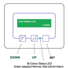
During normal operation the display will show G.M.Treble Ltd along with the current system pressure.
