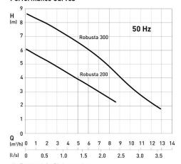
H = Total head; Q = Discharge volume Curves to ISO 9906 (60 Hz available on request)
