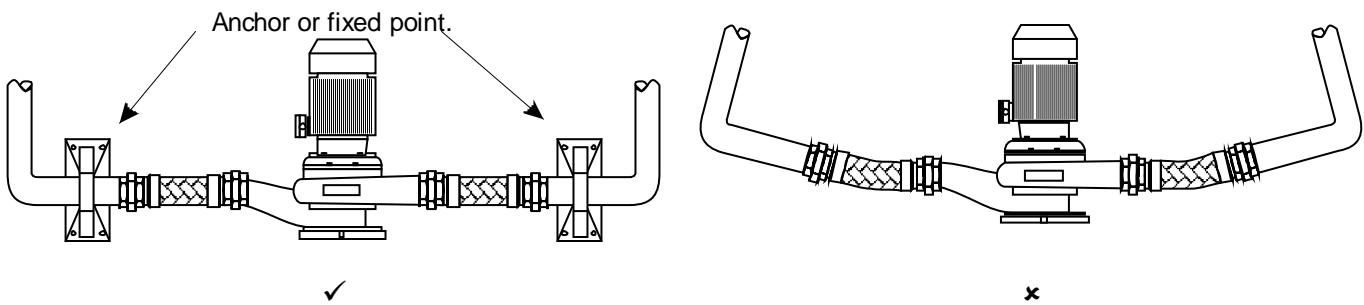
Stainless steel pump connectors will exert a pressure thrust in service and must be anchored to protect adjacent pipework and equipment. Rubber bellows will extend under pressure and must be anchored to prevent this happening.
