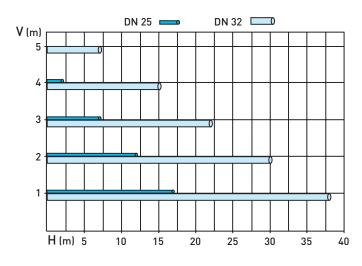
Maximum pipe length allowable for the optimum functioning of the unit. Allowance has been made for two 90° bends and one Sulzer non-return valve.
