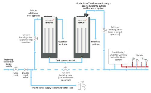
Additional storage tanks must be the same capacity as the main TankBoost unit.
